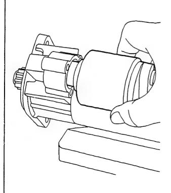
Disassembling solenoid switch
